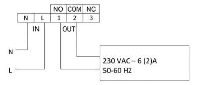
The voltage at the terminals No.1 and No.2 depends only on the controller system, the wire size is determined by the type of device to be controlled. The thread length is not relevant, the receiver can be installed near the boiler or far from it, but not installed under the housing of the boiler.
